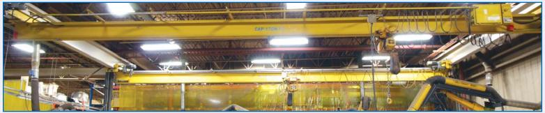
(2) PROTECH 1.5 TON single girder underslung overhead bridge cranes with approximate 37.5 ft. span, KITO 1.5 TON underslung hoists with pendant control
