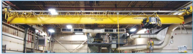
PROTECH 7.5 TON single girder underslung overhead bridge crane with approximate 37.5 ft. span, R&M SPACEMASTER SX 7.5 TON underslung hoist with pendant control s/n 915-22-A
